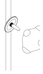
Gently thread pendant onto the stem. Be sure to carefully place the pendant so as not to damage the lamp during installation..
