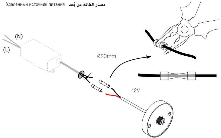
**EN** Output, connect positive wire to positive 12V and negative wire to negative 12V. Input, connect live to live (L) and neutral to neutral (N).
