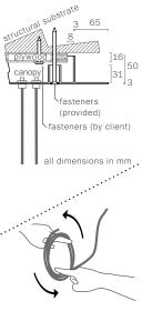
Connections from the plywood to the structural substrate are the client's responsibility.
