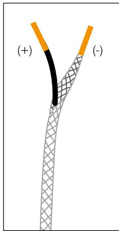
**EN** For multiple pendant installations, ensure that the braided outer wires are all connected to one 12V output wire and all inner insulated wires are connected to the other or a short will occur.
