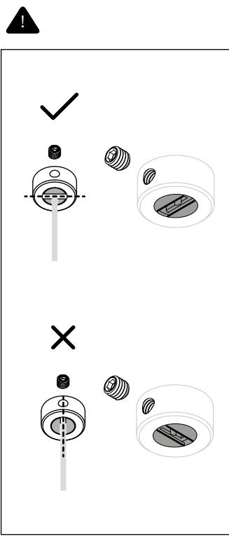
**EN** Do not overtighten! Perform a gentle tug test to ensure the coaxial cable is secure.
