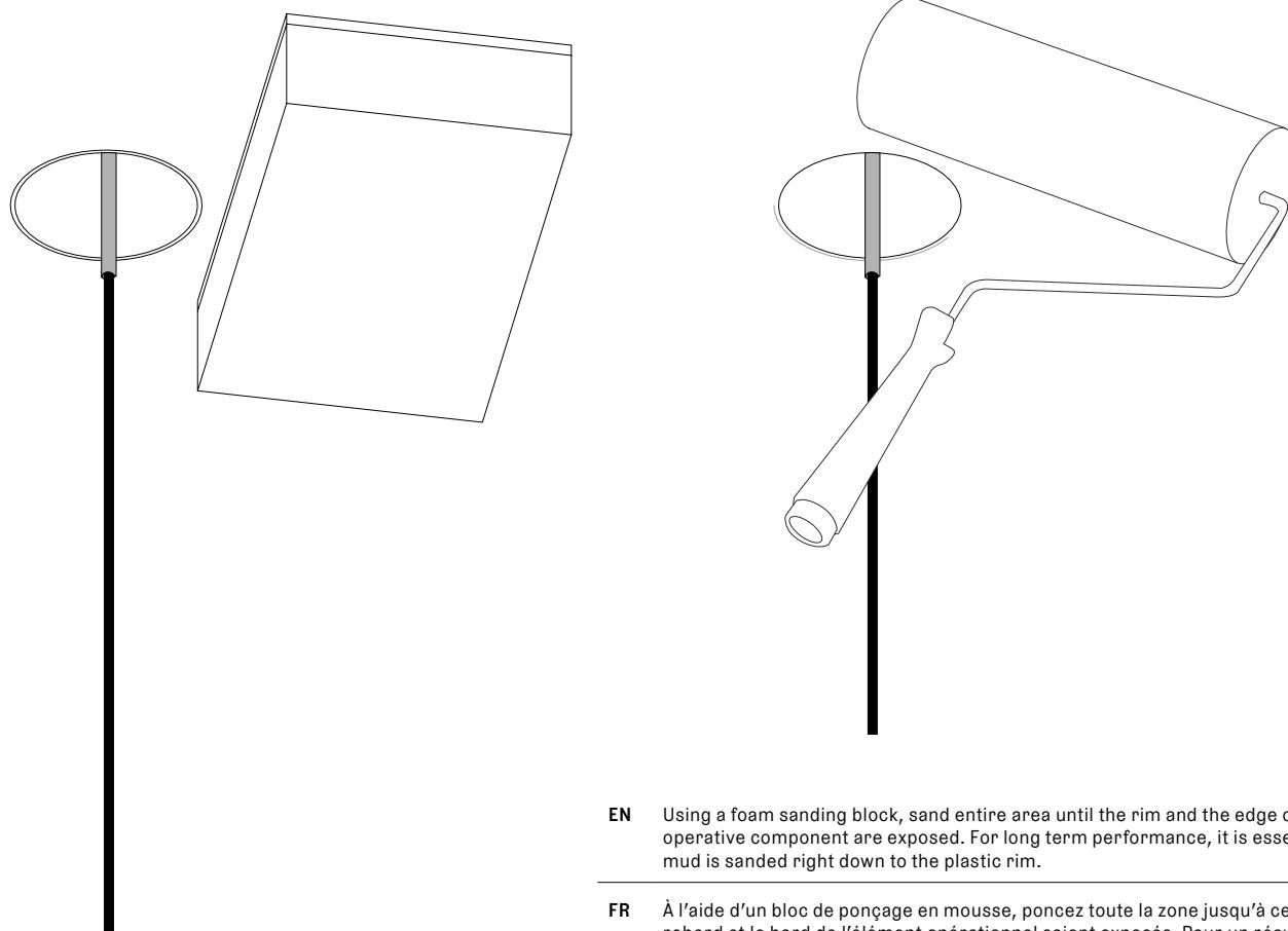
**EN** Using a foam sanding block, sand entire area until the rim and the edge of the operative component are exposed. For long term performance, it is essential that mud is sanded right down to the plastic rim.
