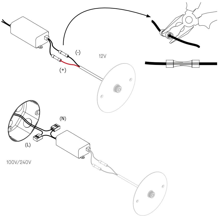
**EN** Connect positive wires to positive 12V and negative wires to negative 12V.
