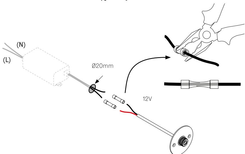
**EN** Connect positive wires to positive 12V and negative wires to negative 12V.
