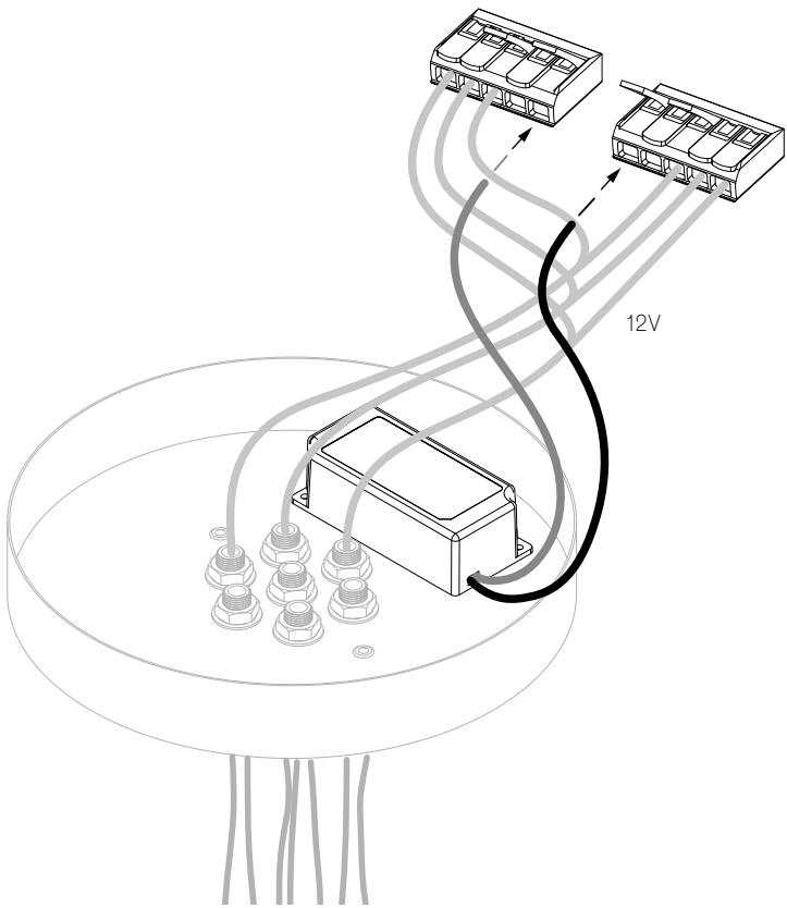
**EN** Connect braided wires to negative 12V and insulated wires to positive 12V.
