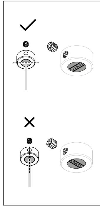
**EN** Do not overtighten! Perform a gentle tug test to ensure the coaxial cable is secure.
