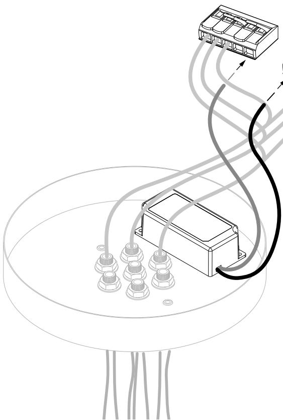
**EN** Connect braided wires to negative 12V and insulated wires to positive 12V.
