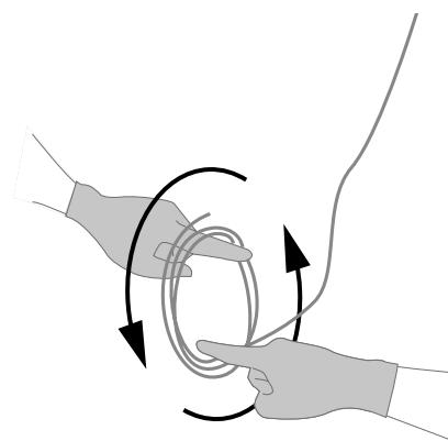
**EN** To avoid kinks, uncoil the coaxial cable in a spool-like manner. Allow the cable to uncoil completely before installing.
