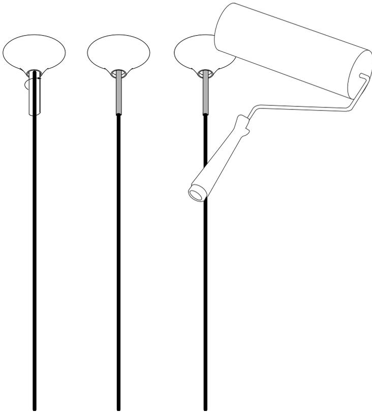
**EN** Use silicone caulking to fill the seam between the ceiling and the canopy. Mask the coaxial cable off with painters tape to help with cleanup. Paint over entire assembly.
