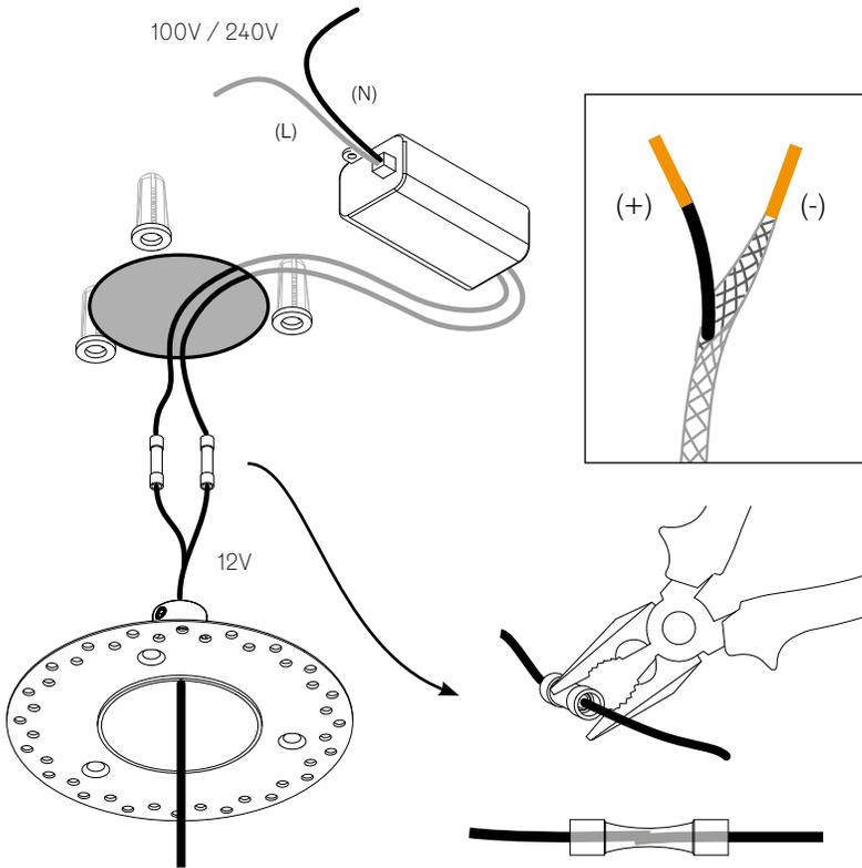
**EN** For multiple pendant installations, ensure that the braided outer wires are all connected to one 12V output wire and all inner insulated wires are connected to the other or a short will occur.
