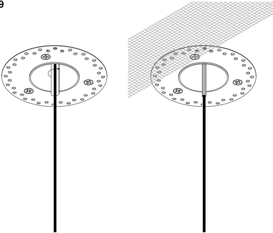
**EN** Mask the coaxial cable off with painters tape to help with cleanup. Tape the mounting plate edges with fiber mesh drywall tape.
