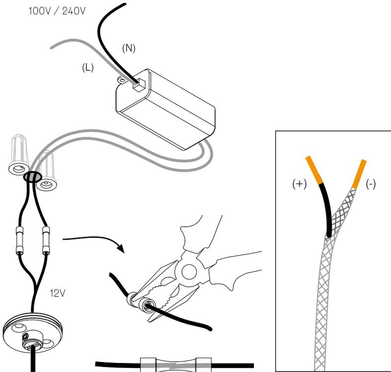
**EN** For multiple pendant installations, ensure that the braided outer wires are all connected to one 12V output wire and all inner insulated wires are connected to the other or a short will occur.
