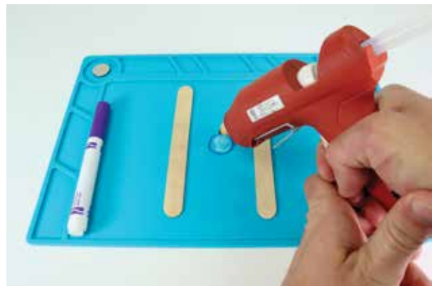
Squeeze hot glue onto the center and stop once it spreads to the edge.
