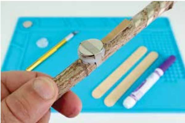
The battery holder creates a flat spot on a rounded wand stem.
