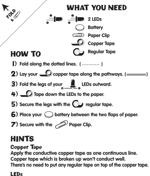
The long legs are Positive and the short legs legs are Negative. They need to match up with the Positive and Negative from the battery.
