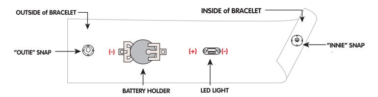
Markings on the Battery Holder & LED indicate Positive (+) & (-) Negative ends. Be sure to arrange as shown: Positive end of battery holder towards the positive end of LED.
