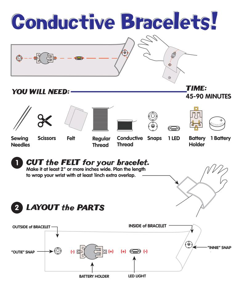
Markings on the Battery Holder & LED indicate Positive (+) & (-) Negative ends. Be sure to arrange as shown: Positive end of battery holder towards the positive end of LED.
