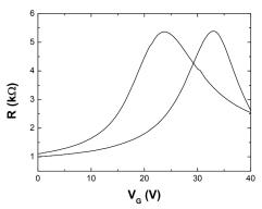
Transfer curve under back gating measured at source-drain voltage of 20mV at room temperature and vacuum conditions.
