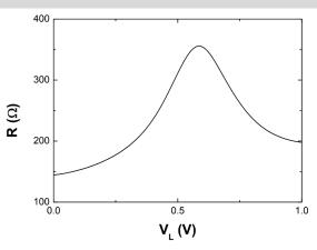
Transfer curve under liquid gating through Phosphate Buffered Saline (PBS, pH=7.3), using the on-chip electrode as gate electrode.
