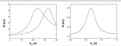
Left: Transfer curve under back gating measured at source-drain voltage of 20mV at room temperature and vacuum conditions. Right: Transfer curve under liquid gating through Phosphate Buffered Saline (PBS, pH=7.3), using the on-chip electrode as gate electrode.
