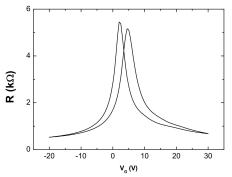
Transfer curve measured at source-drain voltage of 20mV, at room temperature and vacuum conditions on a device with W=50  $\mu$ m, L=60  $\mu$ m.
