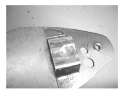
6) IT MAY BE NECESSARY TO GRIND OR SAND DOWN THE EXCESS WELD MATERIAL THAT SUPPORTED THE LAMP SOCKET AS SHOWN IN FIGURE 6. DO SO BY USING A DREMOL OR EQUIVALENT. THE RAISED BRACKET SHOULD BE AS SMOOTH AND FLAT AS POSSIBLE FOR PROPER MOUNTING OF THE CUSTOM LED FLUSHMOUNT INSERTS.
