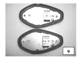
7) DRILL A SMALL 1/16" PILOT HOLE IN THE RAISED METAL BRACKET AS SHOWN. THE HOLE SHOULD BE AS CENTERED AS POSSIBLE SIDE-TO-SIDE, AND SLIGHTLY TOWARDS THE FRONT (FATTER END OF THE LP FM III).
