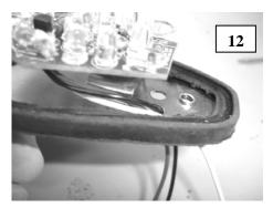
10) INSERT THE PROVIDED SCREW THROUGH THE MOUNTING HOLE IN THE CUSTOM LED FLUSHMOUNT INSERT. INSTALL THE NYLON SPACER ON THE BOTTOM SIDE OF THE FLUSHMOUNT INSERT AS SHOWN.
