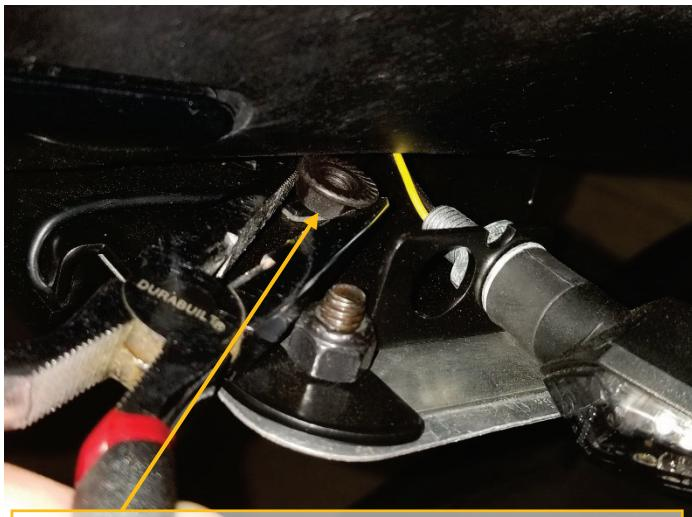
**11)** Position the bracket on the two bolts, and fasten with the provided nuts. It may help to use a needle-nose to position the nut while you turn the bolts.
