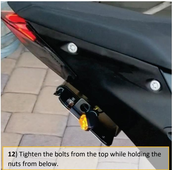
**12)** Tighten the bolts from the top while holding the nuts from below.
