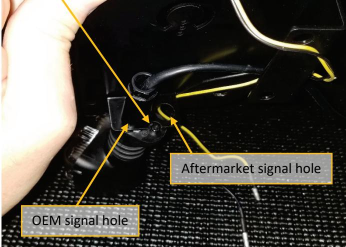
**9)** Pass the connectors/wires from the plate bracket through the grommet.
