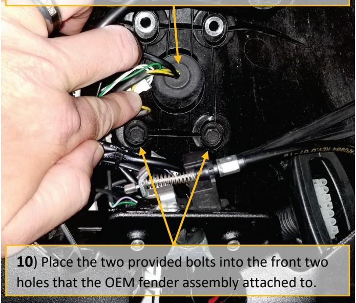
**10)** Place the two provided bolts into the front two holes that the OEM fender assembly attached to.
