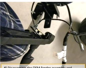
4) Disassemble the OEM fender assembly and extract the sub-harness which branches off from the 4-pin connector into a left-turn, right-turn and license plate light connector.
