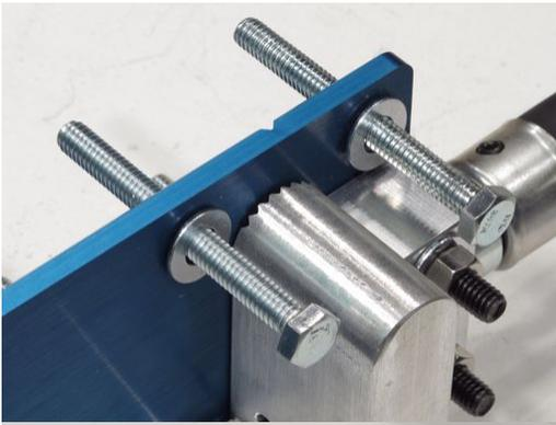
Next place a washer and the other two long bolts through the other set of holes, and tighten.
