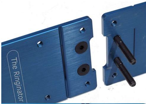
Next, take the two long cone bolts and pass them through the cutting plate. This is where the arbor holder mounts.
