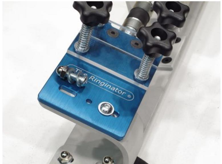
The cutting plate attaches next. Use the 1" button head bolts. Place a washer on each side. The entire assembly slides so you can line it up with your drill. After it is lined up, tighten the bolts.
