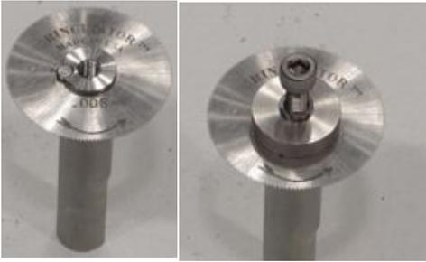
The blade goes on to the end of the arbor. Make sure the notch in the blade lines up with the pin. This prevents the blade from slipping under high cutting loads.
