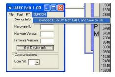
UAFC has enough non-volatile EEPROM memory for saving up to 27 minutes of datalogging. By accessing the "EEPROM" menu item you can down datalogs stored in UAFC EEPROM to disk in "CSV" format. This data can be easily imported into Microsoft Excel, the data field separator is a comma ",".
