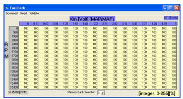
This screen allows you to edit the your 256 point Fuel Correction Table, yellow area. The blue area is the MAP/MAF Axis (X Axis), you can not directly edit it in this screen, it must be edited in the Globals screen. The grey area is the RPM Axis (Y Axis), you can not directly edit it in this screen, it must be edited in the Globals screen.
