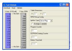
Settings in the Fuel Globals screen are applied to all 3 memory banks. After downloading new Global settings to UAFC you must cycle power to UAFC for the settings to take place.
