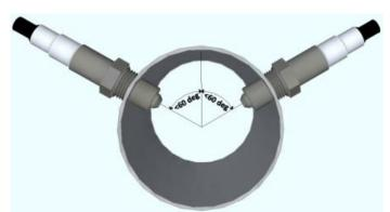
allow gravity to remove water condensation from the sensor.
