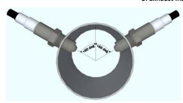
The Lambda sensor should be installed between the 10 o'clock and the 2 o'clock position, less than 60 degrees from vertical, this will allow gravity to remove water condensation from the sensor.
