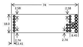
All dimensions in mm. All pinheader pitch is 2.54mm.
