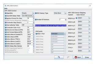
Set "EGO Sensor Type" to "Wide Band". Set "Number of Sensors" to appropriate number of Lambda sensors.
