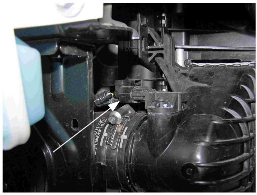
**13.** Next locate the MAP sensor connector on the right side and disconnect it.
