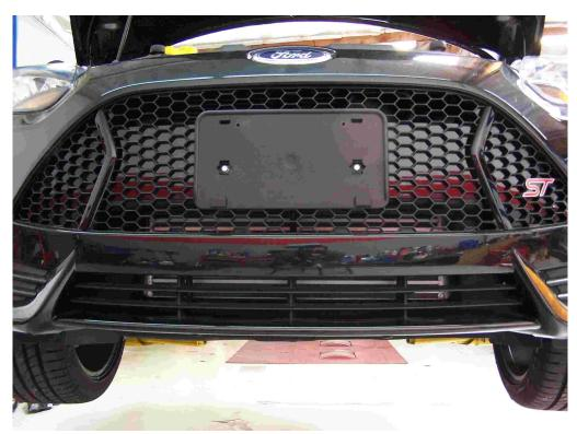
**35.** Reinstall the front bumper, headlights and all other components in reverse of removal to complete your installation.
