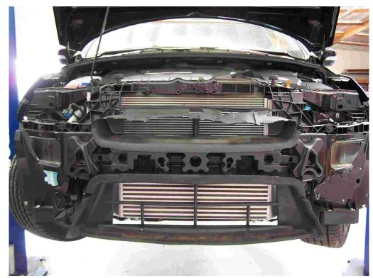
**34.** Next install the upper and lower rubber shrouds in reverse of removal. **Note:** While we recommend using the lower rubber shroud it's not required. If you desire, keeping it out will show more of the intercooler once the bumper is installed.
