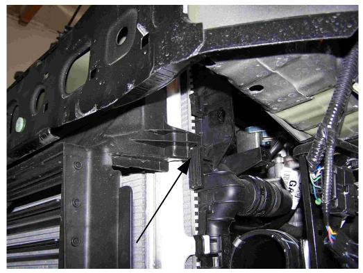
**18.** Lift the active grill shutter system up and out of it's rail and remove it completely, there's two mounting points on each side.
