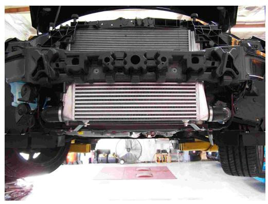
$\textbf{33.} \ \ \text{Next install the plastic bumper beam in reverse of removal}.$
