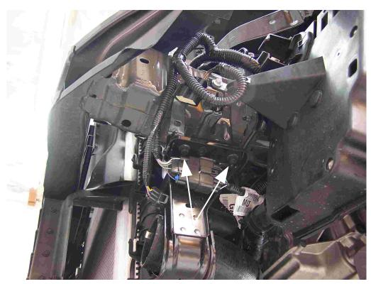
**17.** Next prepare to remove the active grill shutter system by loosening the two radiator support bracket bolts **(do not remove them completely).** This will allow the radiator to drop down just enough to lift the active grill shutter system upward and out of its tabs. Once the grill shutter is removed tighten the radiator support bolts back to 15ft lbs.
