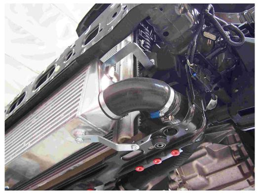
**28.** Once the intercooler is aligned torque the four bolts into the intercooler and the two bolts going through the radiator to 15ft lbs. Next torque the smaller 6mm bolts on the lower bracket to 7ft lbs.
