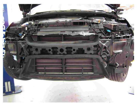
**11.** Bumper cover properly removed. **Note:** Sometimes the front plastic license plate holder will be riveted through the bumper and into the plastic bumper beam, if that's the case you must drill out the rivets for the bumper to release.
