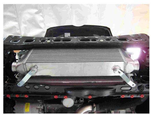
**25.** Install the two lower brackets as shown with the supplied hardware, again do not fully tighten.
