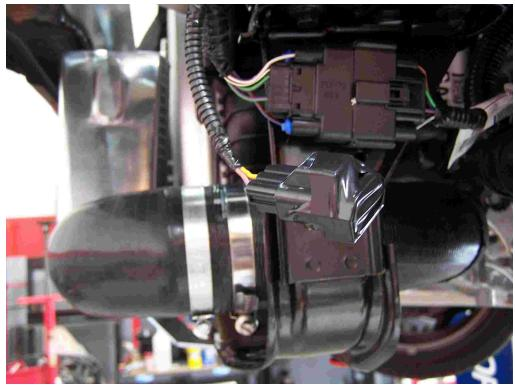
**32.** Use some electrical tape to cover up the connecter which will stay open from the active grill shutter system, you can use a ziptie as well to keep it from hanging.
