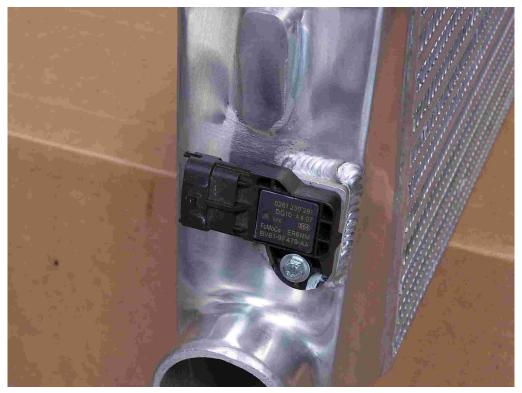
**20.** MAP sensor installed correctly using the supplied hardware.
