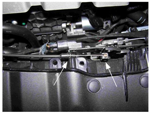
**7.** Pry out the hood latch cable from the latch assembly using a screw driver or pliers.
