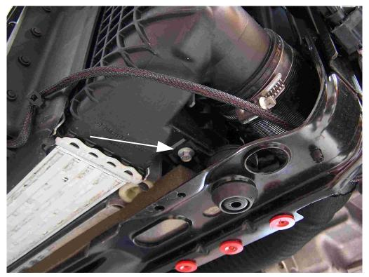
**15.** Next locate and remove the two bolts securing the intercooler to the radiator, one on each side. Once you've done that you can remove the intercooler by simply rotating it forward and slipping it downward and out.
