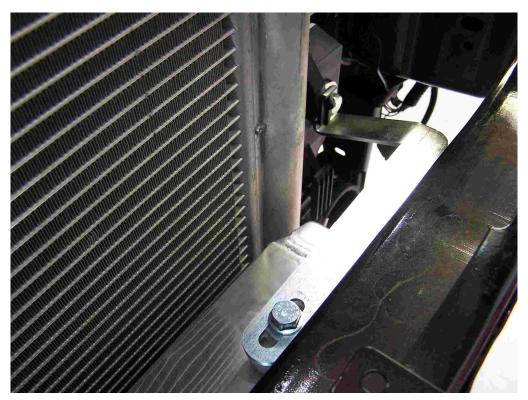
**23.** Using a hydraulic jack to aid in holding the intercooler, center the intercooler on the radiator with the brackets and install using the supplied hardware as shown. The large washer and locknut fit on the backside of the radiator, snug the hardware but do not tighten fully for final adjustment.
