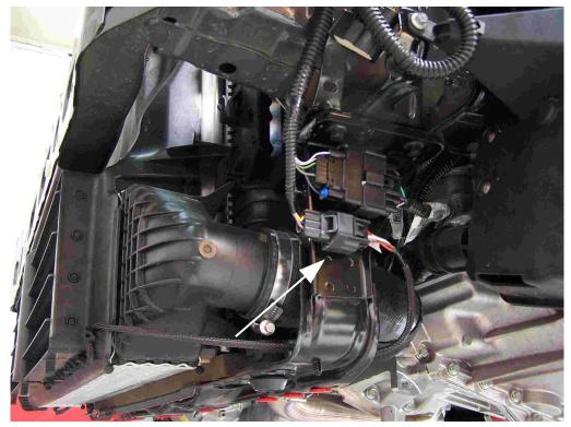
**16.** Locate the active grill shutter electrical connector and disconnect it, also remove it from the radiator support so it can be removed in the next few steps.
