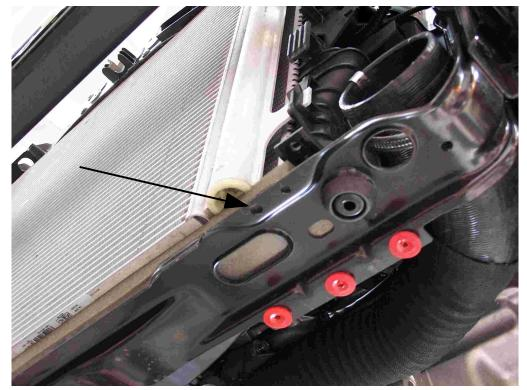
**24.** Next locate the two holes on the radiator support, this is where the lower bracket will attach with the supplied hardware, **(only the larger of the two holes will be used)**, see arrow.
