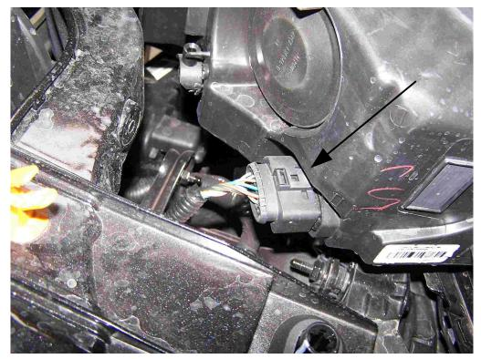
**6.** Disconnect the electric plug behind both headlights.
