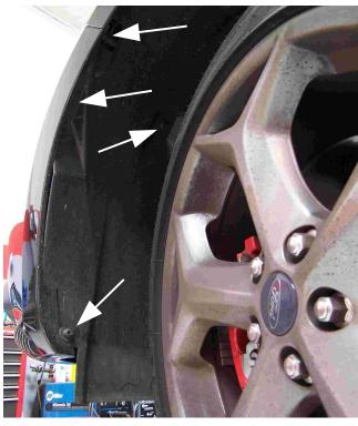
**3.** Remove the three T-30 Torx fender liner screws and one plastic clip from the bumper, pull back fender liner to expose the plastic bumper to fender guide.
