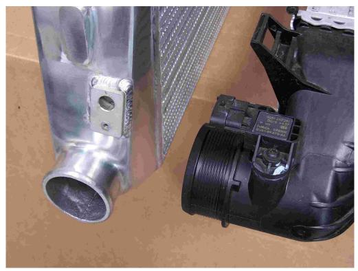
**19.** Remove an reinstall the MAP sensor from the stock intercooler into the FSWERKS intercooler using the supplied hardware. Using a small amount of lube on the o-ring before assembly is recommended.
