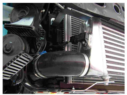
**31.** Reconnect the MAP sensor wiring harness, you'll have to remove the plastic clip which is connected to the A/C hose otherwise the harness will not reach.
