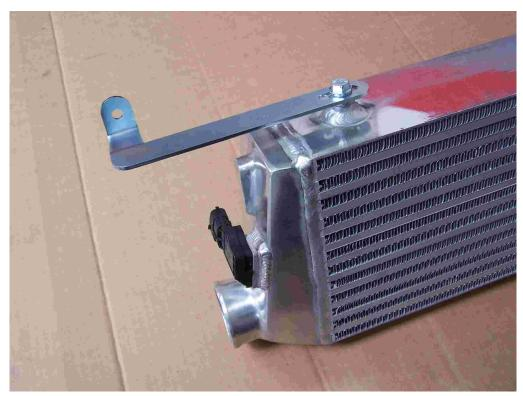
**21.** Next install the supplied upper two brackets on the intercooler as shown, do not tighten the hardware as they will need further adjustment later. Do this on both sides.
