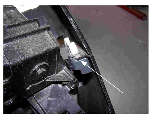
**9.** Loosen the two bolts on the bumper to fender guide approximately one turn, then using a small flat screwdriver gently pry where the arrow illustrates, this will allow the bumper to pull out and away from the fender.
