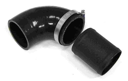
**29.** At this point you can start installing the silicone into the aluminum tubing as shown. **Note:** The ninety degree silicone is short on one end and longer on the other, ensure that the short end connects to the aluminum tube as shown.
