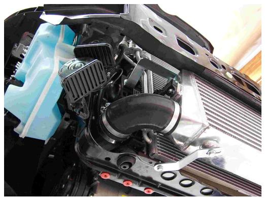
**30.** Next using the supplied hose clamps install both ninety degree silicone hoses into the factory rubber hose and onto the intercooler as shown, (the stock hose clamps will be reused from the factory rubber hoses). Ensure that there's proper clearance for the silicone and rubber hoses between the radiator and radiator support bracket, any rubbing can cause damage in the long run, adjust as neccessary. Tighten all six hose clamps.
