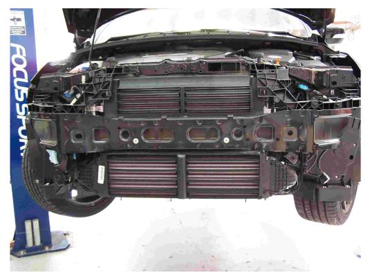
**12.** Remove the upper and lower rubber shrouds, the upper one simply pulls off two tabs, the lower one is held in place with two T-30 Torx screws. Next remove the plastic bumper beam which needs the release tabs to be squeezed.
