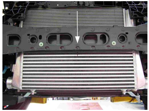
**26.** At this point measure out the center point on the intercooler and make a mark as shown, using the FORD logo which is stamped into the metal bumper beam as a center point align the intercooler from left to right.
