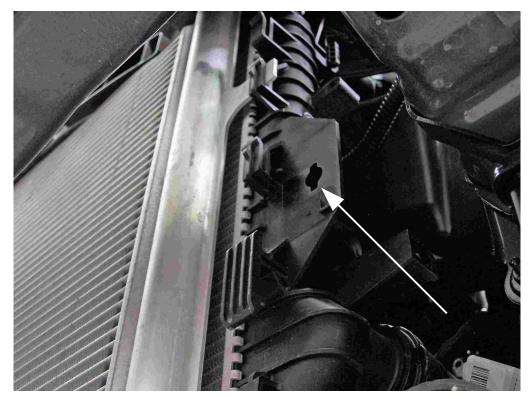
**22.** Locate this hole on the radiator, this is where the two upper intercooler brackets will fit with the supplied hardware.
