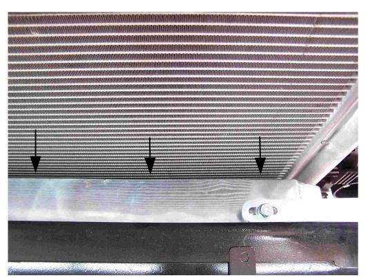
**27.** Be mindful of the space between the condensor and the intercooler and make sure it's straight from left to right on both the top and bottom. There should be approximately 1/2" or more clearance on both top and bottom.
