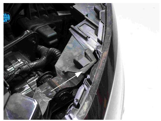
**10.** Pry plastic tab where arrow illustrates to release the bumper cover and gently remove bumper cover.
