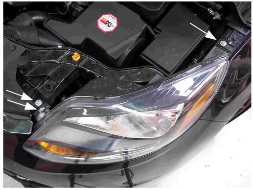
**5.** Locate and remove the two T-30 Torx screws securing the two front headlights, pull lights upward and forward to remove. Also remove the other two T-30 Torx screws securing the grill.
