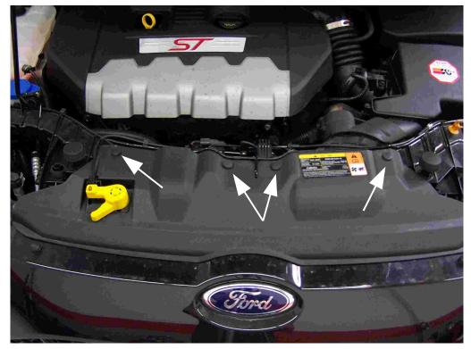
**8.** Using a small flat screwdriver remove the four plastic snap clips above the grill.
