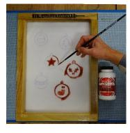
Step 3) Raise the edges of the screen away from the table by placing a wedge, such as a coin under each corner. Using a fine brush paint the screen filler around the outlines.
