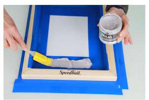
Apply a generous amount of Akua™ Carborundum Gel to the top of your screen. Make sure the gel spans the entire width of the screen mesh.
