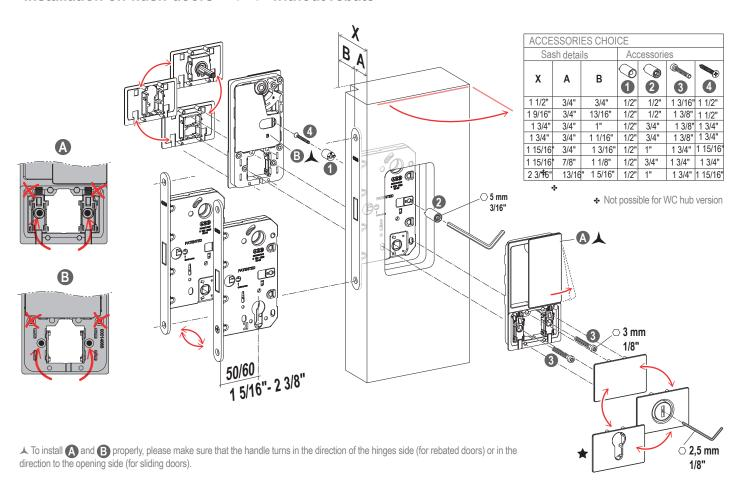
★ Block the cylinder only after the handle fastening and the cover application
