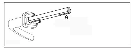
The square should go through the hole in the latch or lock and be positioned with the retention screw slot at the bottom.
