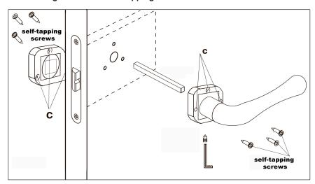
Drill pilot holes for self-tapping screws with a diameter of 1/16" (no more than 5/8" deep).
