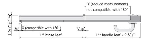
(B): if the handle leaf<sup>(1)</sup> is less than 15 3/8" wide, Y<sup>(2)</sup> must also be reduced.
