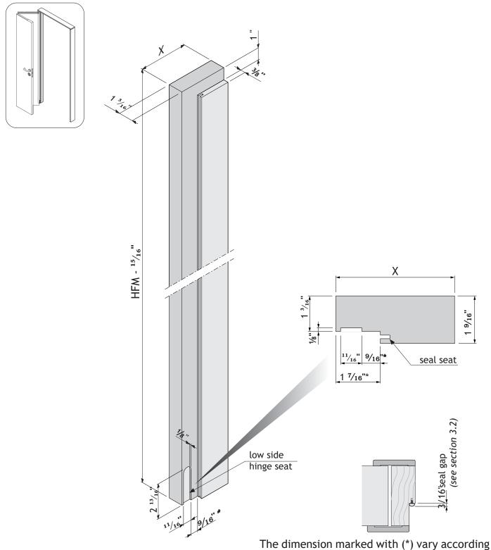
The dimension marked with (\*) vary according to the seal gap dimensions
