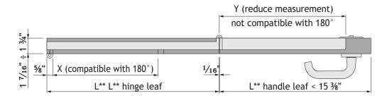
(\*\*) Hinge leaf and handle leaf widths are calculated with a reciprocal distance of 1/16"
