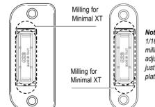
Note. When Easy-Fix XT 1/16" is inserted into the milling of the Minimal XT, the adjustment can be obtained just turning the tray, not the plate.
