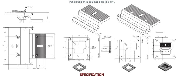
MATERIAL: Extruded Aluminum Alloy 6063, tempered to T5, the screws are mild steel with a zinc coating
