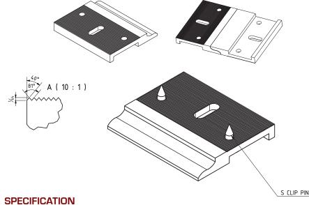
MATERIAL: Extruded Aluminum Alloy 6063, tempered to T5, the screws are zinc coated mild steel
