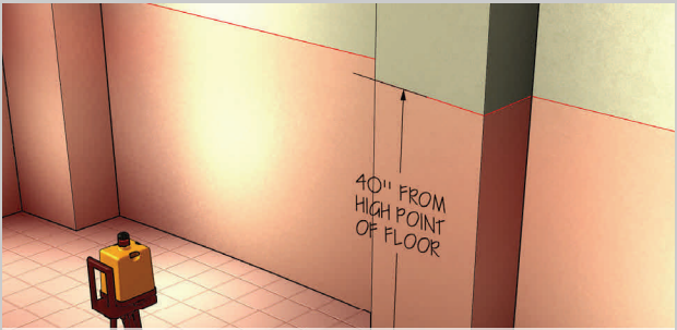
Find high point of floor, set horizontal bench mark 40" above bottom panel.
