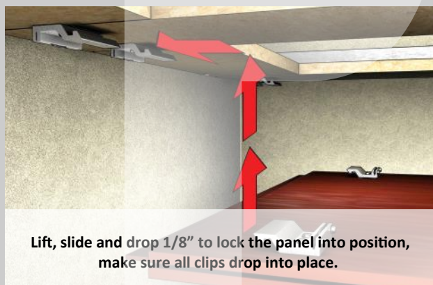
Check for alignment, slight side-to-side adjustments can be made by adjusting the clip.
