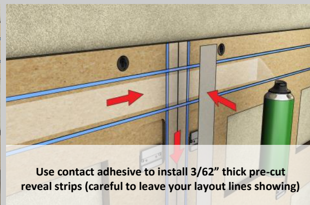
Layout the position of the reveals on site, adding 1" to the width of the chalk line + the width of the reveal
