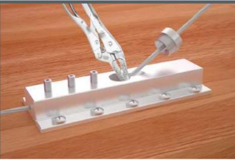
Carefully lift the panel into position from a secure platform. Install the Cloud Hangers to the cables, unscrew the friction ring and feed the cable through horizontal locking hole with needle nose pliers. Clamp the 1/8" cable with needle nose vise.
