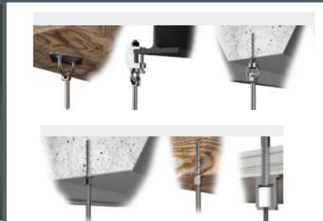
Examine the ceiling structure above and determine if the cable connection points are workable. If required adjust the location of the template to locate solid connection points.
