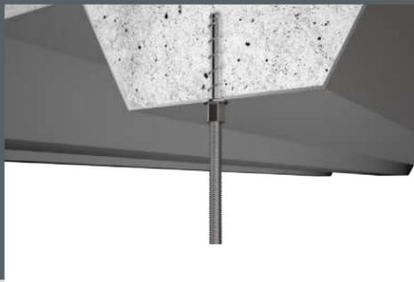
Finished sheet rock ceiling and hidden concrete deck, use a 1/4" - 20 Concrete Bolt connected to a threaded rod. SEE Step 12.
