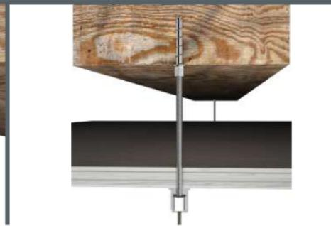
Cloud Hanging, Ball Connector & 5 Ft. 1/8" Cable Clamp connected to a threaded rod. There should be a few inches of the threaded rod exposed through the finished ceiling. After the ceiling is finished the exposed rod is cut to 3/8" below the ceiling and cleaned up, ready for the Ball Connector.
