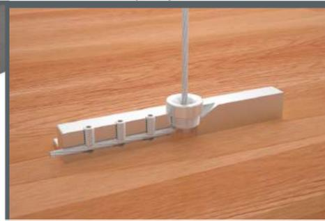
Cut of cable off flush with the end of the Cloud Hanger. The 1/8" stainless steel cable is difficult to cut, use a large pair of wire cutters or small bolt cutter.
