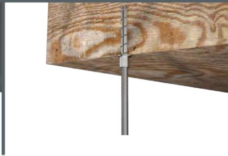
Finished sheet rock ceiling and hidden wood beam, use a 1/4" - 20 Concrete Bolt connected to a threaded rod.
