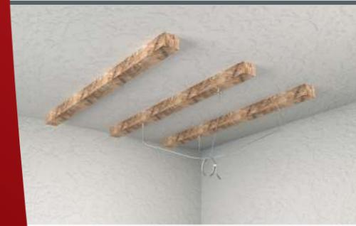
Install the structural connections & cables. The cables should be dropped about 12" below the final panel level. Tie the cables together well above the work zone.
