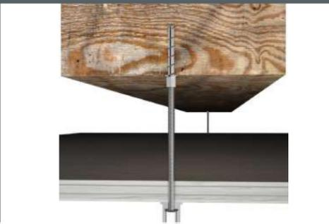
Finished sheet rock ceiling and hidden steel beams, use a 1/4" - 20 Beam Clamp connected to a threaded rod. There should be a few inches of the threaded rod exposed through the finished ceiling.
