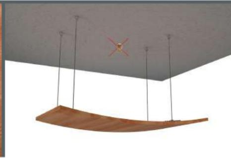
Take a good look at the panel from the ground to make sure it does not hit anything. And does not block HVAC Vents, Fire Sprinklers or other critical equipment. Note, A fixed cable connection should not be used if the panel will be constantly subject to sway or noticeable movement from HVAC vents, fan or any other source.
