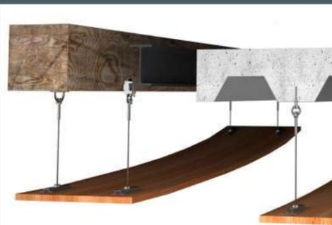
There are three common ceiling structures that the Cloud Hanging is suspended from, steel beams, concrete and wood.
