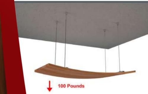
While standing solidly on the ladder pull down firmly on all the cable connections. If properly connected the ends should show no signs movement of failure with 100 pounds of added force.
