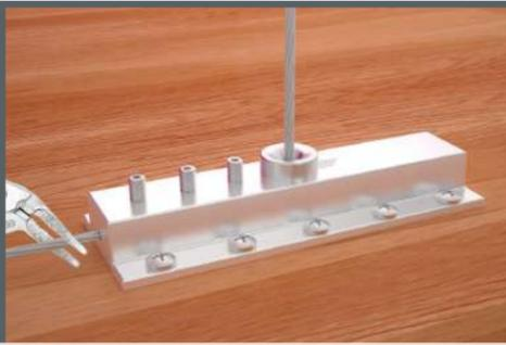
Reinstall the friction ring and tighten all 3 of the cap screws onto the cable. Use the needle nose vise grips to adjust the cable length until the Cloud is at the correct height. Tighten all three set screws to lock the cable in place. Use a firm force to lock all 3 cable lock cap screws in place, however, not enough to cut the cable.
