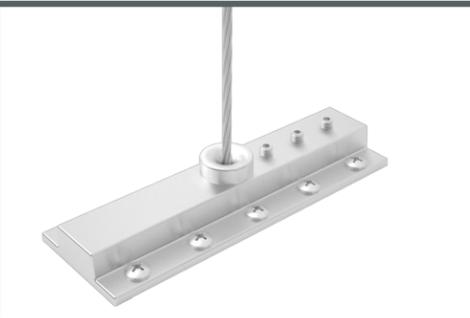
Install the Cloud Hangers onto the Cloud Panel. There are 10 screw holes drilled for #8 x 3/4" pan head wood screws, use all the screws.
