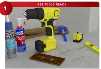
Required Tools: 760 Countertop Bolt, 765 Ball End Allen Wrench, 770 Countertop Router Template, 915 Router Bit, 3/32 Offset, Small Battery-Operated Drill, Silicone Adhesive, Dead Blow Hammer, Denatured Alcohol Spray Bottle.
