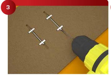
A 765 Ball End Allen Wrench and a small battery operated drill can be used to tighten the bolt in a second. (**Tip:** Use the lowest torque setting on the drill.)
