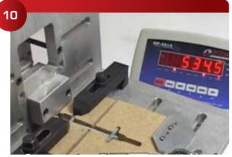
(**Tip:** Be careful to not over-tighten the bolt, particle board will break at approximately 500 pounds of tension. These are Grade 5 bolts rated for 2000lbs.)
