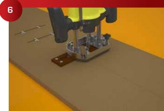
The template is screwed to the underside of the countertop. A plunge cut 1/4" Router is used with any standard 1/4" Shaft, 1/2" Ball Bearing with a 3/32 Offset.
