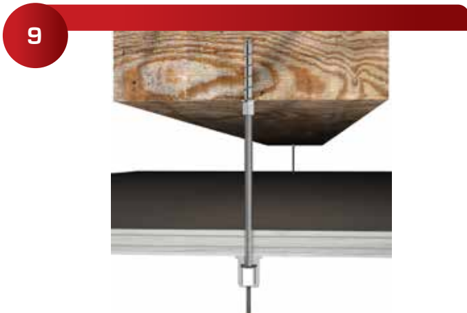
When working with finished sheet rock ceiling and hidden steel beams. A good option is to use a 610 Cloud Hanger, 1/4"-20, Beam Clamp connected to a 1/4"-20 threaded rod left exposed through the finished ceiling. After the ceiling is finished the exposed rod is cut to 1/2" below the ceiling and cleaned up, ready for the 620 Ball Connector. SEE step 12
