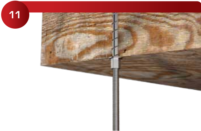
When working with finished sheet rock ceiling and hidden wood beam . A good option is to use a 612 Cloud Hanger, 1/4"-20, Screw Anchor connected to a threaded rod.
