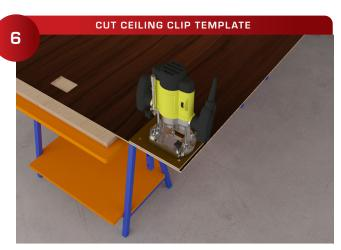
Cut a ¼" thick full size Plywood Template for each size of panels. Use the small 539 Router Template to cutout the clip pockets in the Plywood Template to locate the placement of every clip pair. Clip placement does not have to be precise.
