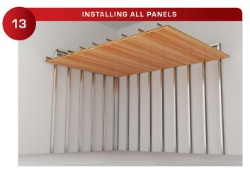
Finished ceiling panels can be glued with a small spot of silicone to hold reveal tolerances. The panels can be removed with enough force to loosen or break the locking arms, this should not damage the clips and the locking arms are replaceable.
