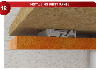
When satisfied with the fit, install the locking arms, and push the panel into place. There should be an audible click when locking arms spring into place. The locks do not have to be installed on every clips, we recommend using locks around the perimeter.
