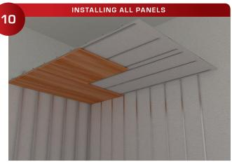
The ceiling clip allows for about ¼" of movement. (**Tip:** The ceiling panel can be glued with a small spot of silicone to hold reveal tolerance.)
