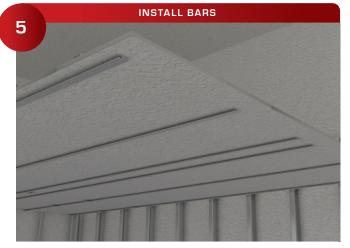
Install the 511 Ceiling Clip Bars, shim if needed to a plate plane. Use 2 screws at bar joints. (Recommendation: Hilti Self Drilling, Self-Tapping Screws at every stud.)
