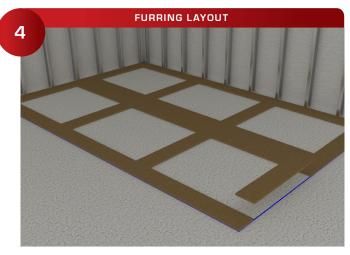
Cut the <sup>3</sup>⁄<sub>4</sub>" plywood furring to fit layout.
