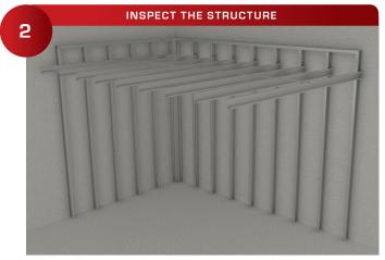
**FIRST:** Insure that the structure above the sheetrock will support the panels you are planning to install. Our weight holding for screws is based on using 16-gauge steel studs.
