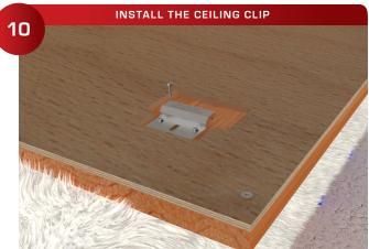
Install the panel 2" Ceiling Clip carefully against the front of the template, with 3 screws.
