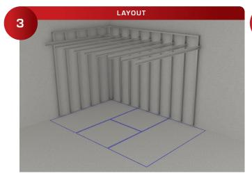
Lay out the perimeter of the panel's layout lines on the floor, to check fit.
