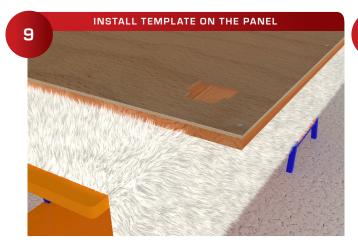
Temperately set the ¼" plywood template panels with a few screws.
