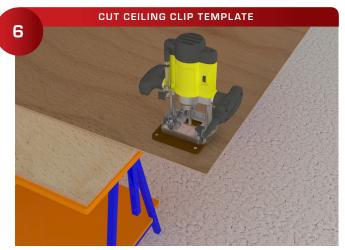
Make a template from ¼" plywood to provide accurate installation of the clips. (**Useful Accessories:** Star Hanger sells the 537 Ceiling Clip Router Template.)
