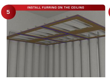
Securely install <sup>3</sup>⁄<sub>4</sub>" plywood furring with a string line, level & flat.
