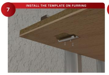
Temperately set the ¼" plywood template in the exact location of the panel with a few screws. Install the 3" Ceiling Clip carefully against the back of the template, with 3 screws.
