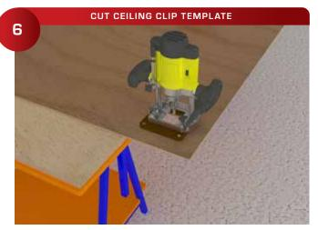
Make a template from 1/4" plywood to provide accurate installation of the clips. (Useful Accessories: Star Hanger sells the 537 Ceiling Clip Router Template.)
