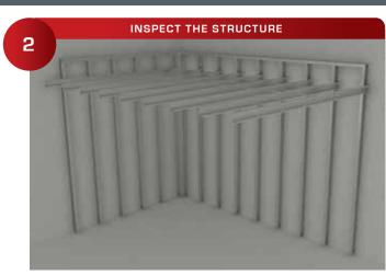
FIRST: Insure that the structure above the sheetrock will support the panels you are planning to install. Our weight holding for screws is based on using 16-gauge steel studs.
