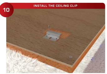
Install the panel 2" Ceiling Clip carefully against the front of the template, with 3 screws.
