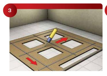
Full size furring sections can be pre-glued and shimmed into place.
