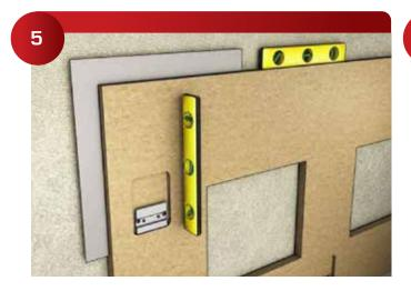
Level and square the corner furring sections with shims and screws as required.
