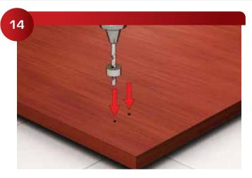
Pre-drill with a 1/16" drill on the back side of the panel at each location mark.
