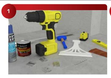
Required Tools; 420 S Clip, 421 S Alignment Clips, Panel Adjuster, 1/32" plastic laminate, Spray Contact Cement, Panel Adhesive.
