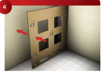
Install the corner furring sections to the field control lines.
