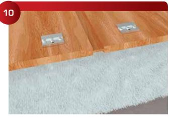
The reveals strips are generally used with bars, either a spline or a dado at back of the panels or both work well. A dab of silicone on the center clip helps hold the panel in place.
