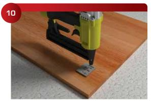
Screw or staple the 400 NZ Clips in the position indicated by the Alignment Clips. (**Tip:** You have the option of using only the center slotted screw if you need the clips to be adjustable.)
