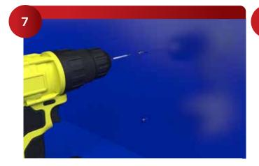
Predrill with a 1/8" Hole. Install stainless steel screws into the fiberglass.
