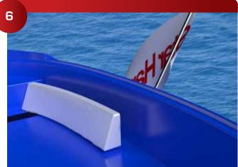
Carefully align the cushion into place and push it firmly to mark the screw positions.
