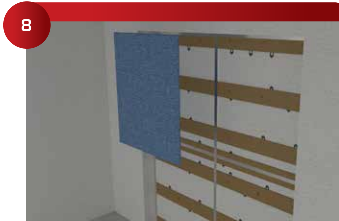
Insert the 229 Galaxy Alignment Pins into the 224 Galaxy.
