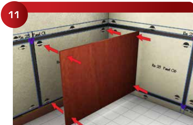
Carefully position your panel over your 211 Alignment Pins and push them firmly to leave a location mark for the 3/16" Mounting Screw.
