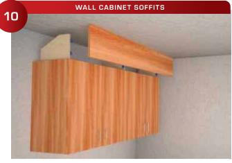
Push the soffit firmly against the 330 Zero Alignment Pins to mark the 334 Mounting Screw locations.
