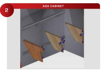
Install both your wall rails with heavy duty self-tapping screws being sure to hit the steel studs. Lock each shop built gusset plate into position and secure each gusset plate with angle brackets.
