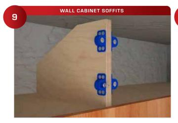
Install the 330 Zero Alignment Pins and press the panels firmly into place to mark the 334 Mounting Screw locations.
